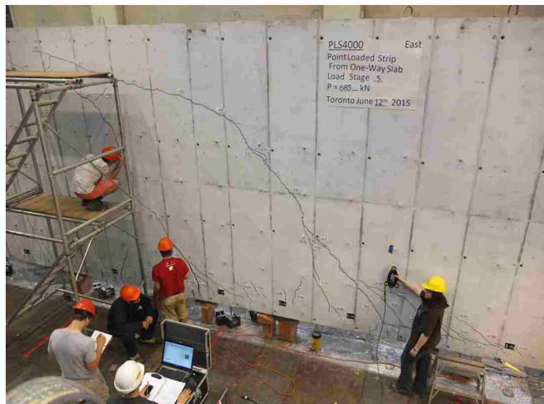
Figure 6.12 – Close-up of shear crack in east side of Toronto beam for phase I
